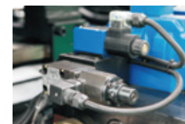
Proportional valve-controlled back pressure
