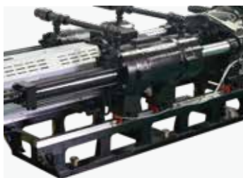
Injection unit support with linear guide rails
